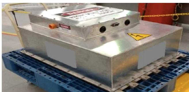
Figure 3: Complete 30kWhr Lithium Ion Battery Pack
