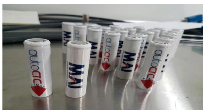
Figure 2: MAI/AutoCRC 18650-type lithium ion battery cells.
